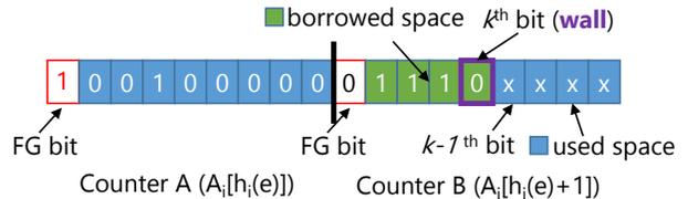
Fig. 1. The ABC framework using bits-borrowing technique.
