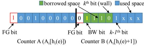
Fig. 2. The ABC framework - bits-borrowing
