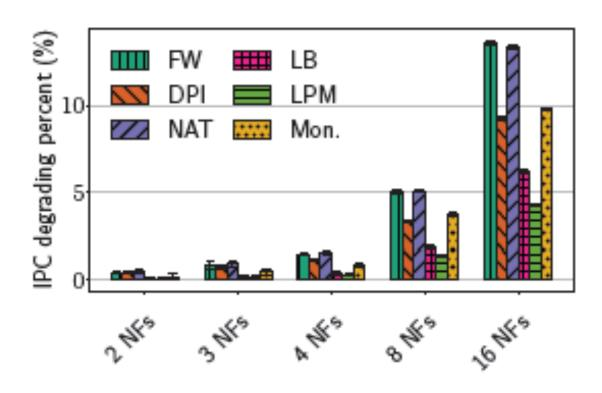
Cache partitioning, and bus arbitration reduce function throughput by less than 13.71% in the worst case.
